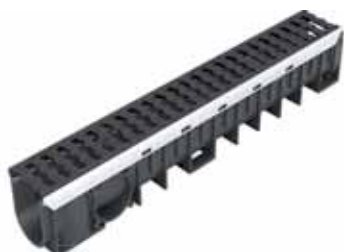
Channel with galvanised steel edge rails with 2 ductile iron gratings DR102DF
