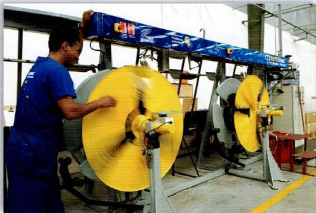
Manufacturing coils on the Buteline Pipewinder
